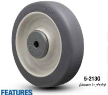
PolyLoc wheels feature a durable grey polyurethane tread mechanically locked to a solid polyolefin wheel core. Tread is molded in, around and through a ribbed wheel core to prevent tread separation (de-bonding) when exposed to
