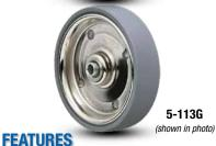
Jarvis welded disc rubber wheels offer designers an attractive alternative for foodservice equipment, medical products, point-of-purchase displays and other institutional applications. These wheels feature a black or grey neoprene rubber tread permanently compressed between two steel discs which are welded together. For improved appearance, the center wheel discs
